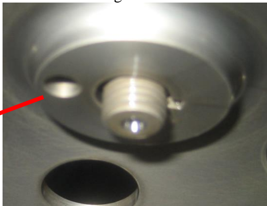
Oil Pump Drive Gear Lock tab retaining slot
