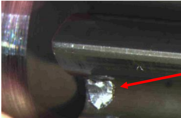
Main Pressure Pump Housing Scoring damage noted
