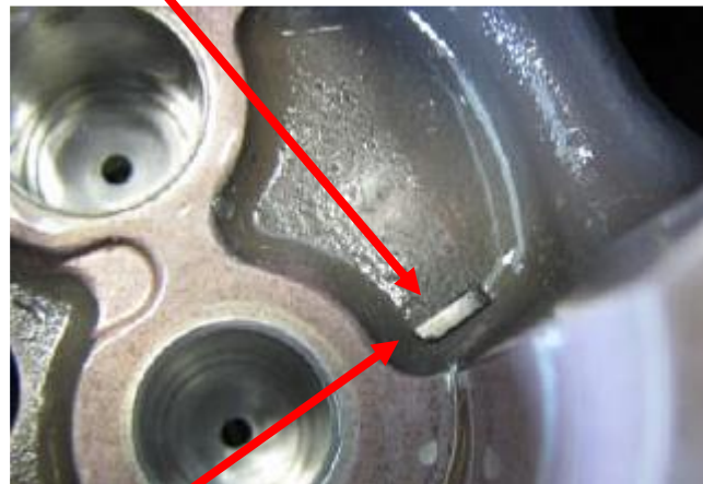
Main Pressure Pump Housing Foreign Debris discovered in housing
