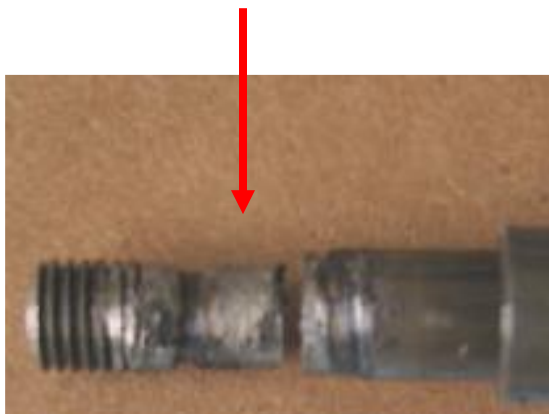
Oil Pump Main Shaft Deformed and fractured
