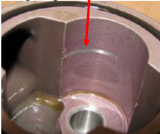
Main Pressure Pump Housing Scoring damage noted
