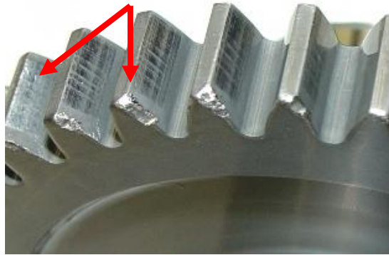
#3 Bearing Anti Rotation Slot Fretting wear with missing material
