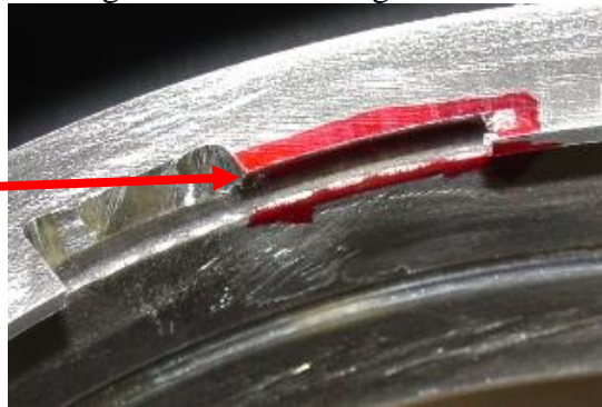
#3 Bearing Anti Rotation Slot Fretting wear with missing material
