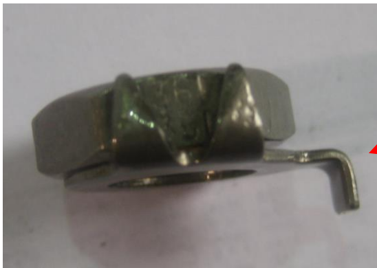
Oil Pump Drive Gear retaining nut Locking tab washer still installed
