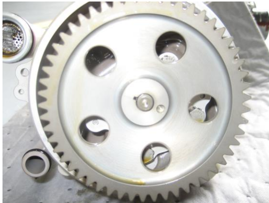
Oil Pump Drive Gear Lock tab retaining slot
