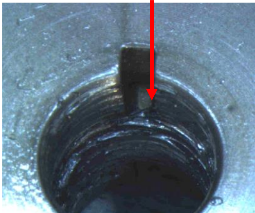
Oil Pump Drive Gear Shaft bore deformed and scored
